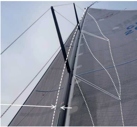
The mast has uncontrolled deflection due to lack of leeward rig tension.
